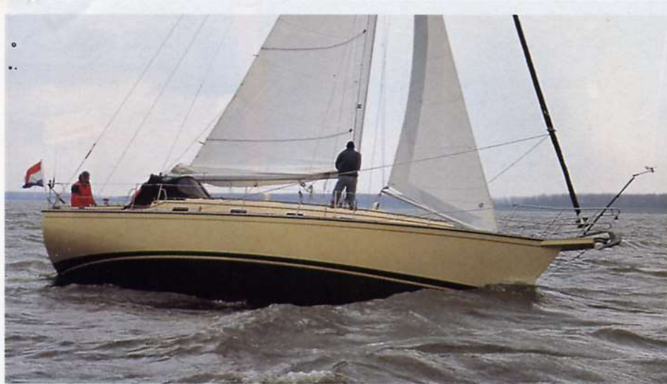
The staysail is set on a boom and is self-tacking, making life easy for the crew in a blow upwind
